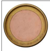
Prototype of a bi-metal coin. Combination of copper-plated steel and Nordic gold.
